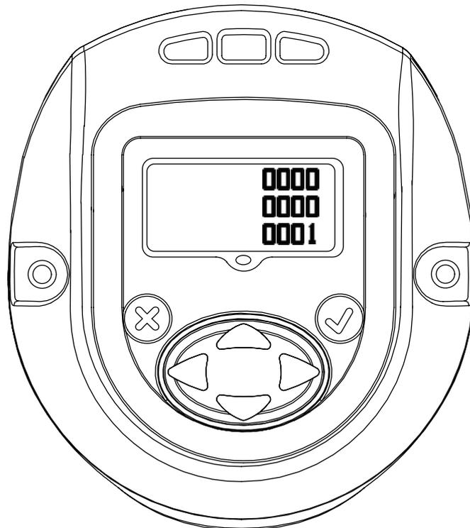
Press the Down key again to return to the Tool ID page. Pressing the right arrow from this page exits back to the password display.
