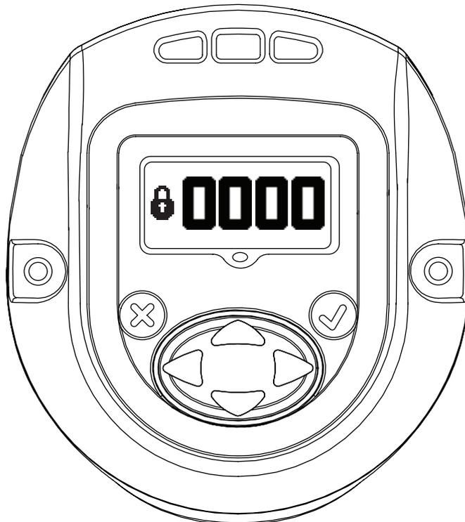
Password can be changed by entering into "EDIT MODE" and using "UP" or "DOWN" key.
