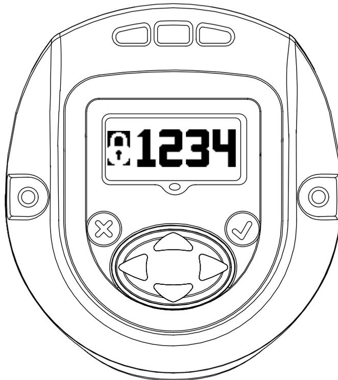
Press 'ENTER' to enter the 'EDIT' mode. Enter the appropriate password to unlock the tool. Press 'ENTER' to exit the 'EDIT' mode.
