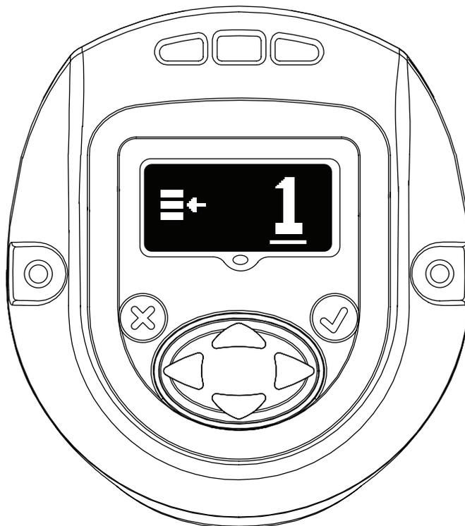
“UP” or “DOWN” key can be used to update the configuration. Pressing “ENTER” again will select the modified configuration.
